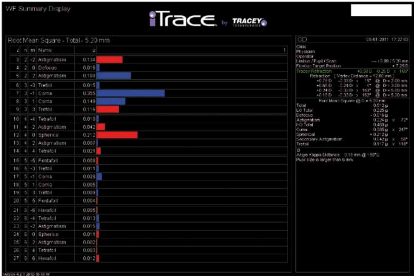
Figure 10. Total RMS values, Total LOA and Total HOA (bottom right) and decomposition in each of the Zernike polynomials represented in red and blue bars depending on the value of the sign.
