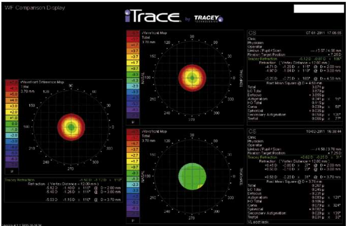
Figure 17. Wavefront Comparison Map Total of a patient who has undergone Lasik refractive surgery. The bottom Wavefront Map (Post Lasik) shows how total aberrations have improved (mainly the defocus), as the map is almost all green (0.0 microns) and to the left, the difference map.
