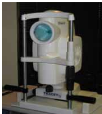
Figure 1. The iTrace measuring system. The latest configuration of the instrument allows aberrometric and topography measurements in the same «measurement axis» for a more real and detailed analysis of the whole ophthalmic optics.
